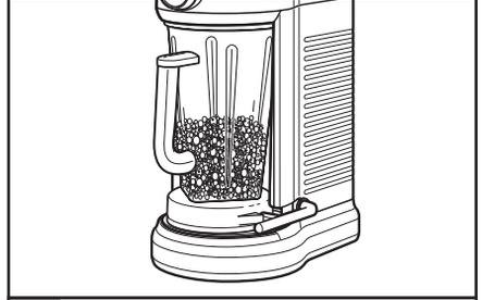
**2 To quickly clean the Blender while in the base:** Add 1 drop of dish soap to half a pitcher of water, and run on the Icy Drinks/Smoothies cycle. Discard water when cycle is finished, and rinse completely.
